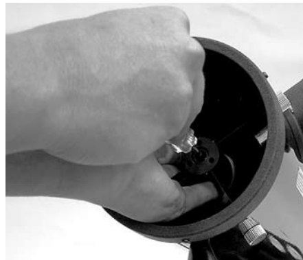
Figure 11. To center the secondary mirror under the focuser, hold the secondary mirror holder in place with your fingers while adjusting the center screw with the Phillips head screwdriver. Do not touch the mirror's surface.
